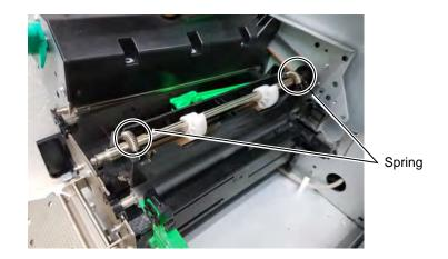
6) Replace the pinch roller upper ass'y with a new one, then reassemble in the reverse order of removal.
