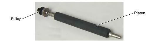
2. When installing the platen, first fully insert the pulley into the printer. Also make sure that the platen holder cover is fixed with the hook.
