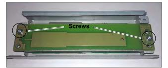
4. Attach the antenna and secure with 2 screws, the proper alignment shown in the figure above.
