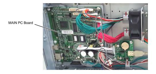
3) Remove the two SMW-3x6 screws, slightly lift and move the MAIN PC board in the direction of the arrow.
