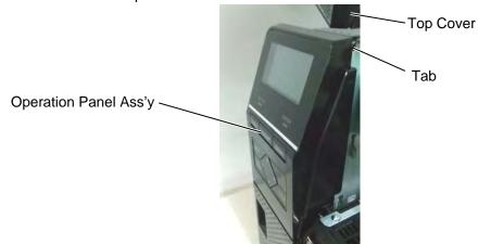
4) Push the operation panel ass'y out through the top hooks direction.
