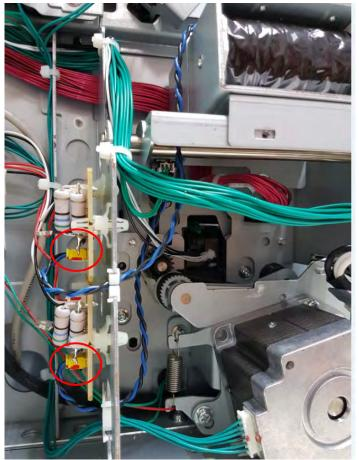
5) Pull the shafts from the Solenoid assembly and remove the Solenoid assembly from the frame. Take note of the spring hook when pulling.
