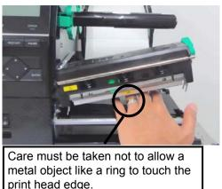
Since the print head element can be easily damaged by shock, please treat it carefully by not hitting a hard object against it.
