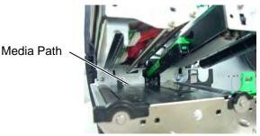
(5) When using the cutter unit, clean the cutter blade and the media path.
