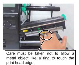
Since the print head element can be easily damaged by shock, please treat it carefully by not hitting a hard object against it.
