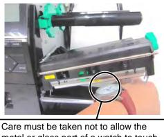
Care must be taken not to allow the metal or glass part of a watch to touch the print head edge.
